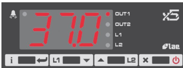
The display shows the temperature readout from the chosen channel (only channel 1 is used on this application). In case of an alarm situation a red light will start flashing in the top left-hand corner of the display. On the right-hand side of the display it is indicated which parameter is shown in the display. Below is listed all possible values and messages that can be shown in the display:
