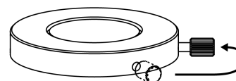
Open Nicol state (mark on the left side) (To fix the polarizer in place, move the fixing screw to another position.)
