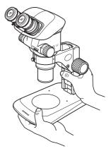
2. The desktop should be a level surface with an inclination of less than 3°, and the load to the microscope should be less than 7 kg (when the SZ2-ST standard stand is used).
