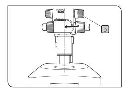
Return the microscope body to the illumination light path by loosening the focusing module clamping knob b, rotating the microscope body gently in the direction of the arrow, aligning visually the objective with the illumination light path and tightening the clamping knob b again. Now the setting of the photo light path is complete.
