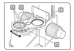
Place the revolving nosepiece mount (c) (with its objective mounts (d) facing upward) where the objective mount has been by aligning the screw holes.
