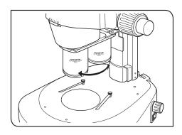
Hold the objective and gently rotate it until a click position on the front, where the objective to be used is engaged in the light path.
