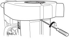
Tightening the screw for epi fluorescence attachment
