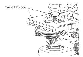
Matching the Ph codes of Ph annular diaphragm and the Ph objective
