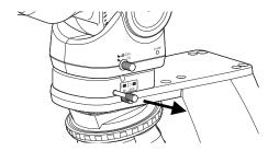
Removing the analyzer from the optical path
