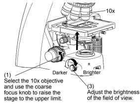
Bringing the 10x objective into the optical path, and raising the stage to the upper limit
