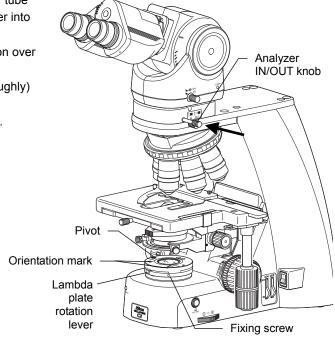
Bringing the analyzer into the optical path Installing the polarizer
