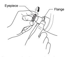
Adjustment using the centering telescope
