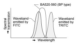
**Band-pass filter** (Only the FITC fluorescent image is visible.)
