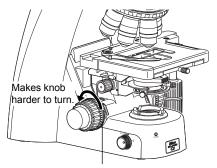
Coarse focus torque adjustment knob
