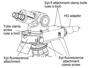
Attaching the epi-fluorescence attachment
