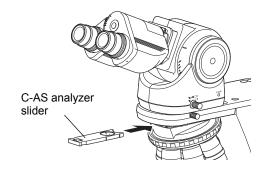
Using D-AS analyzer slider
