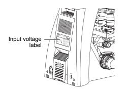
Checking the input voltage
