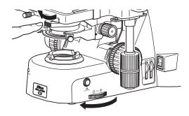
Fully open field and aperture diaphragms.
