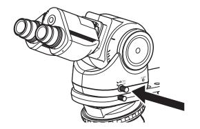
Switching the optical path 100% to the binocular part
