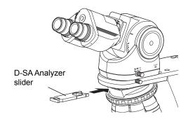
Using D-SA analyzer slider
