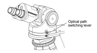
Switching the optical path of the tube
