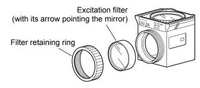
Thickness of filter is ≥6 mm and ≤7.2 mm
