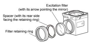
Thickness of filter is ≥3.5 mm and <4.5 mm
