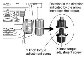
Adjusting the torque of XY knobs
