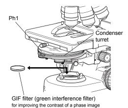
Bring the Ph annular diaphragm into the optical path.
