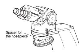
Using the spacer for the nosepiece
