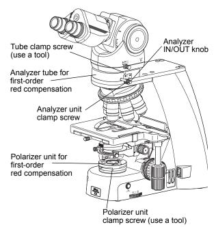
Attaching an analyzer tube for first-order red compensation, and a polarizer unit for first-order red compensation
