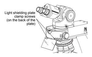
Attaching a light shielding plate
