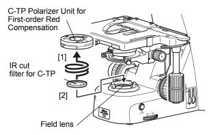
Attaching an infrared ray blocking filter
