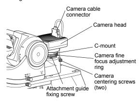
Adjusting the camera head attachment position
