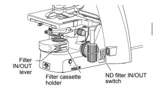
Adjusting the brightness with ND filters
