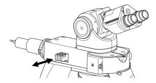
Adjusting the brightness with ND filters
