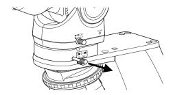
Remove the analyzer from the optical path.
