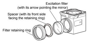
Thickness of filter is ≥4.5 mm and <6 mm
