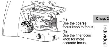
Using the coarse focus knob to focus→Using the fine focus knob for more accurate focus
