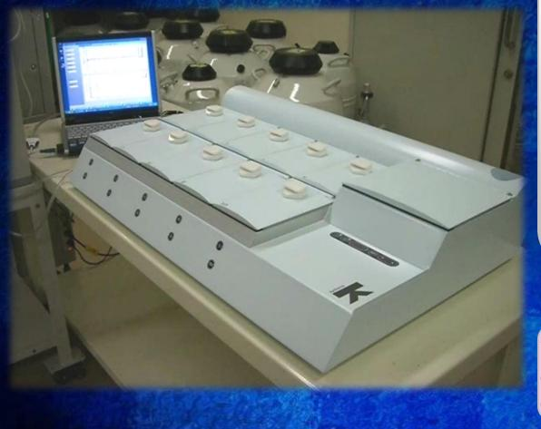
This incubator has 10 individual nonhumidified compartments which differentiates it from other incubators on the market whereas humidified culture condition was fundamental to most of the laboratories at that moment.
